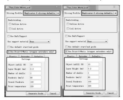
If you want to print dual colors with ABS filament, select Replicator slicing defaults under the Slicing Profile column, and lower the Feedrate to 60 and Travel Feedrate to 80.
