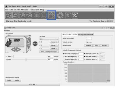
Input the following target values: 220°C for the extruder and 115°C for the heating platform. After entering the values, the platform will start to warm up. When the extruder temperature reaches 50°C, the cooling fan will activate and the current temperature value will display to the right as shown on the following page.
