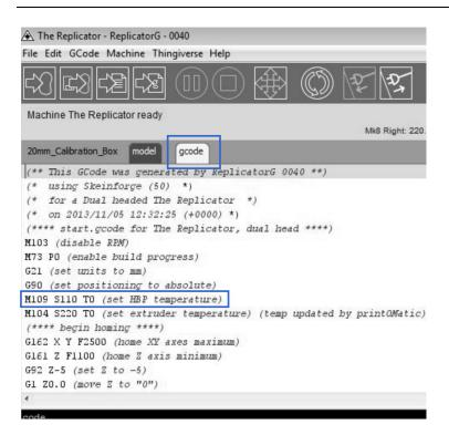
After modifying, click on file and save the sample. Next, click on the left most icon on the green bar, as highlighted below. The Gcode has now been sent to the printer and the object will start printing shortly.
