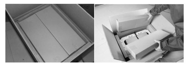
You can see the top of the printer along with more boxes inside. The large box with the black wire is the accessory box. This contains the extruder(s), SD card, and other important components. Do not remove the accessory box and its contents yet. Note: Do not lift the box by the black cable. Doing so could cause damage.
