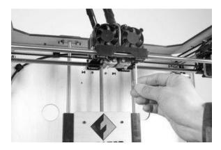
Next is the installation of the filament bracket. If you have two brackets, install one on each side; If you only have one, install it on the right hand side (when viewing the creator from the front).
