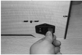
Now plug the USB A to B cable into the USB B-type port, do not plug the other end in yet.
