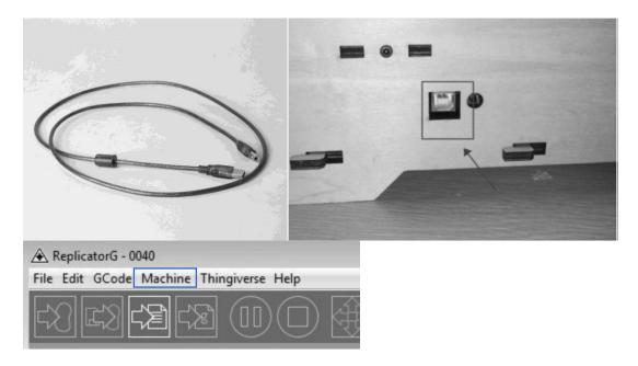
Inside the Replicator G software, click Machine > Connection (serial port) > Rescan serial ports, if no new ports appear, then the software driver has not been installed. To install the driver manually, go to 'My Computer' and right click on 'Properties'. The basic system parameters appear. Next, select 'Device Manager'.
