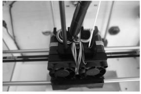
When you have removed the guide tube, you can remove the filament that is inside the guide tube. To avoid any blockages during printing, please ensure that the two threads are loaded from the middle. There are two wire trays, one runs clockwise and the other one runs counter-clockwise, as shown below:
