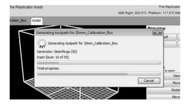
After the Gcode is generated, the temperature of the bottom plate needs to be changed. See below for the required modification. First, select Gcode as shown highlighted in the illustration below and change 'M109 S110 T0' to 'M109 S115 T0'.
