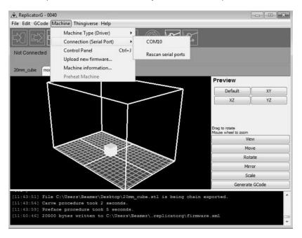
Now we can link the machine to the computer. Click on the printer connect icon highlighted in blue.
